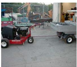
Getting the Aerator out to the greens was always a hassle. So, we made up a towbar. Generally we make things out of what we have laying around, if possible. The towbar was a piece of thinwall rectangular tubing, the hitch a scrap of 1/4 by 2, and a few bolts and some rebar.
